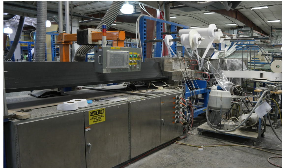
The fiberglass is saturated with resin, in the die, and heat cured in a continuous process
