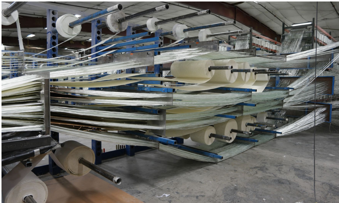
Glass reinforcements are guided into the die
