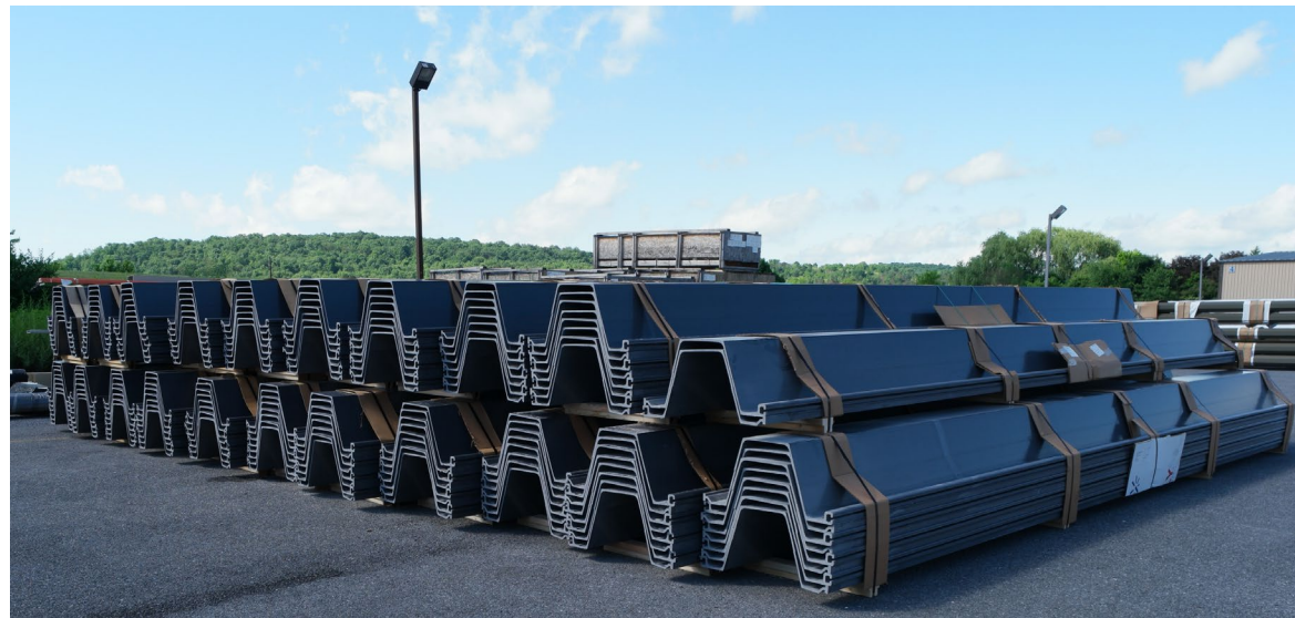
Sheet piles are cut to length and prepared for shipment
