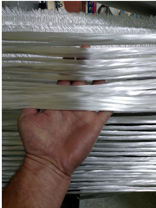
Unidirectional roving make up the bulk of the longitudinal properties
