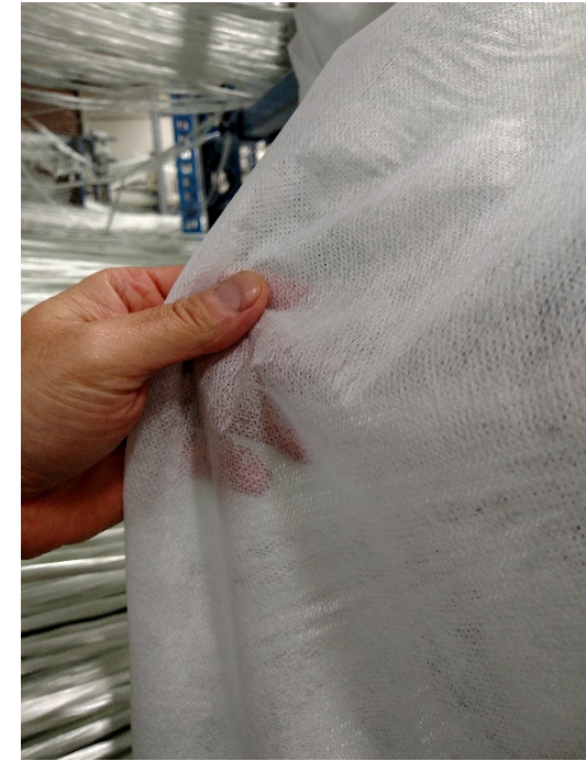
Thermoplastic polyester veils are applied to the outer surface for added UV protection
