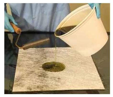
**FRP** – Fiber Reinforced Polymer Industrial fiberglass based on thermoset resin chemistry
