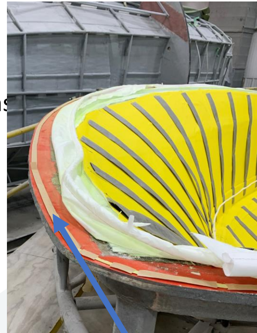
Tacky Tape on 380 LXF Hull
