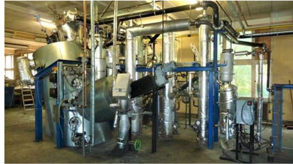
7 ton/day Pilot Thermolyzer (CHZ Technologies)
