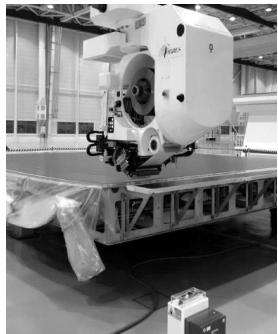
Automated Tape Laying
