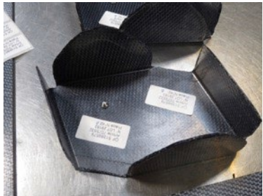
Thermoplastic fuselage clip for Airbus A350. Source: CW
