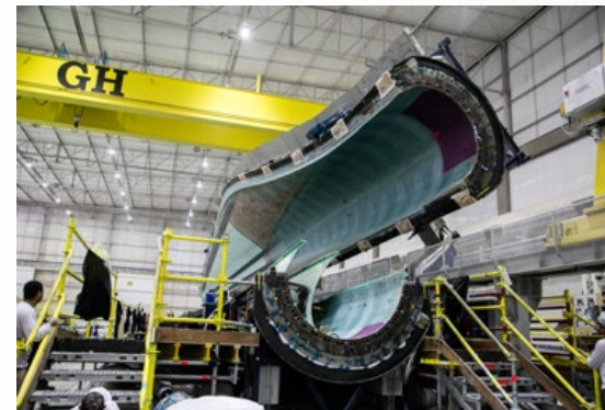
Wind blade mold closing. Source: Aeris Wind Energy
