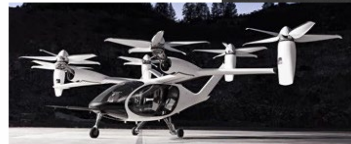
Joby Aviation's unnamed and autonomous tiltrotor eVTOL seats up to two passengers. Source: Joby Aviation
