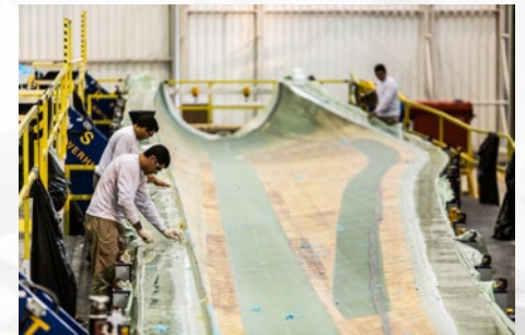
Wind blade layup with balsa core and glass fiber. Source: Aeris Wind Energy
