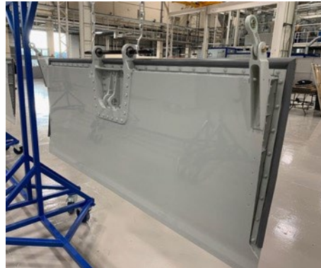
Airbus A320 spoiler, made via RTM in Prestwick, Scotland by Spirit Aerosystems. Source: CW
