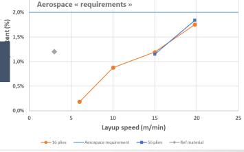
ILSS = 70% at 6m/min - 50% at 20m/min Reference material = 25% at 3 m/min
