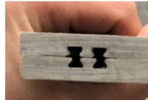
Actual Pultruded Samples made at L&L
