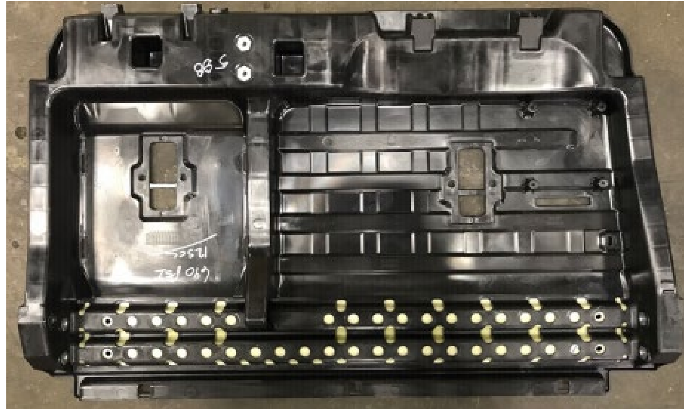
Combining pultrusion where strength needed most + feature integration achieved with injection molded material
