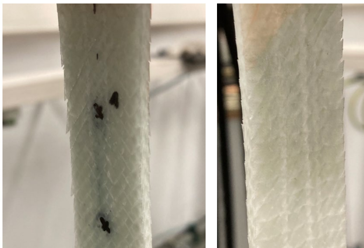
Coupon sample with NDT after 500 load cycles
