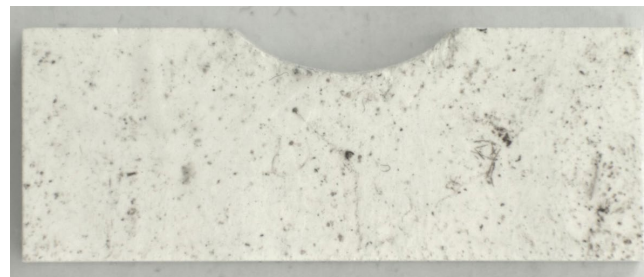
Cutting depth approx. 1,4 mm
