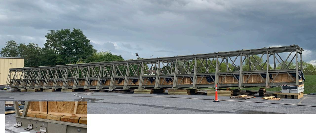
Uniform Load Test - 72psf (dead+live=164,000 lbs ±) without anchorage in CCG yard
