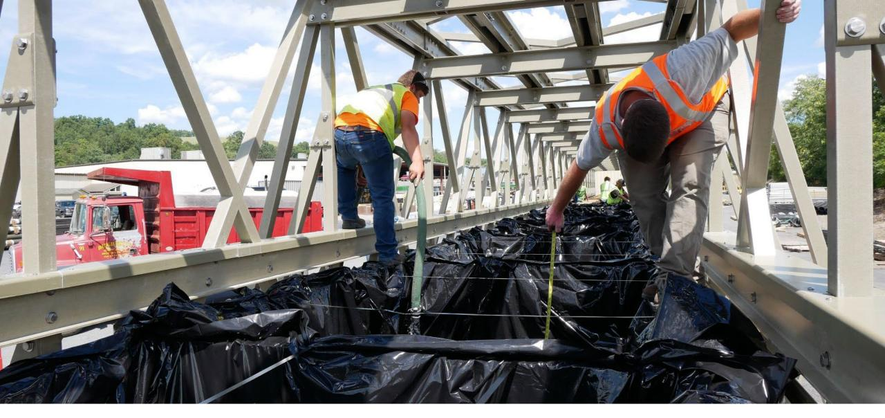
Testing: Utilized water filled pools to safely apply the uniform live load
