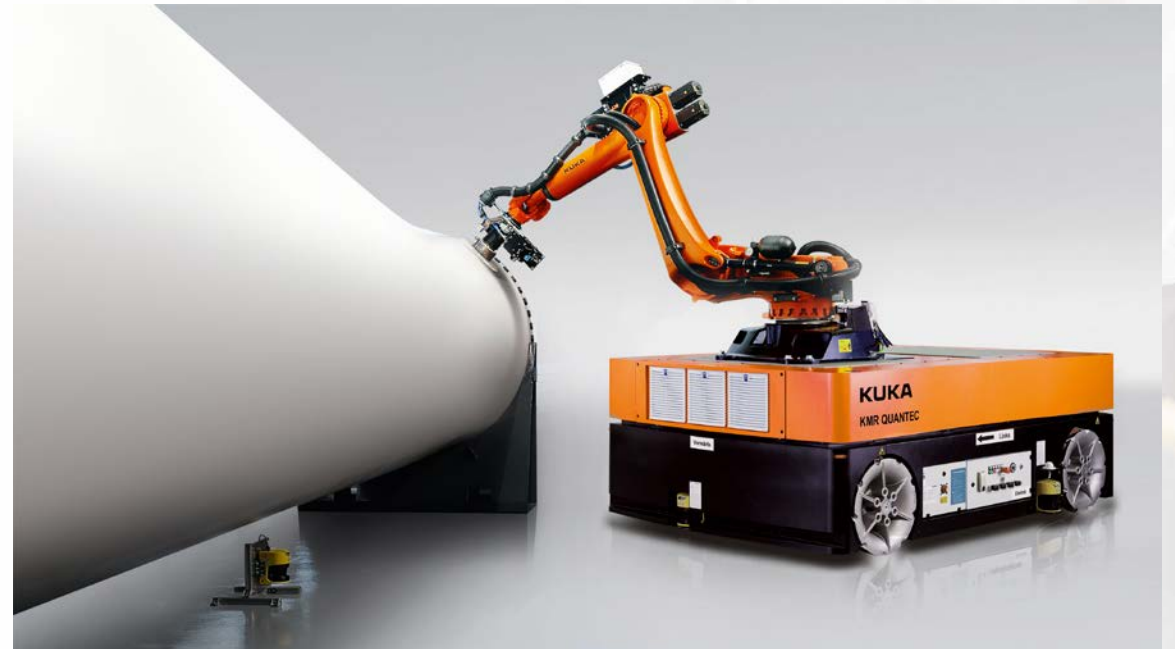
Kuka robotic polishing mobile platform Source: Kuka
