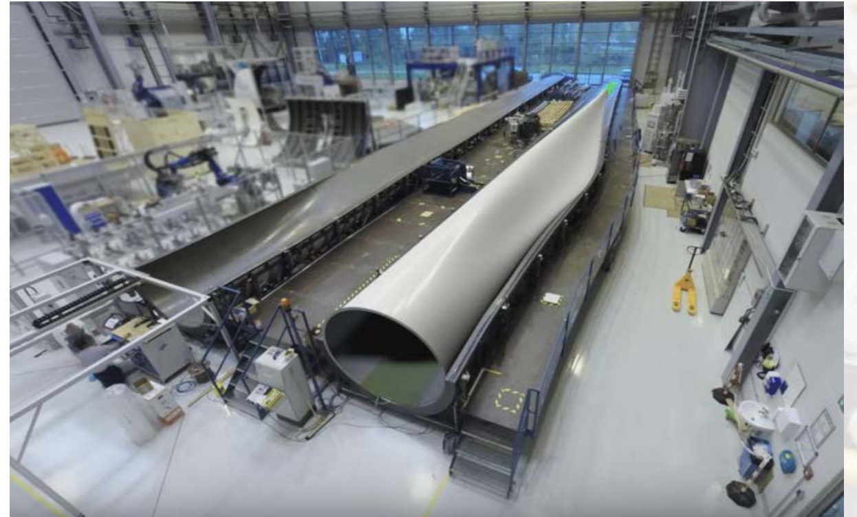
DNV GL Clamshell Molds Source: North American Wind Power
