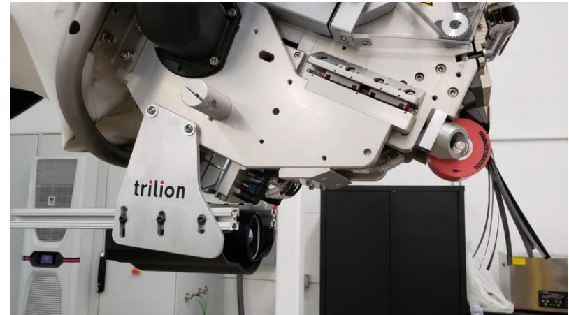
Trillion InSitu NDE system on Joby Coriolis Robot Head.
