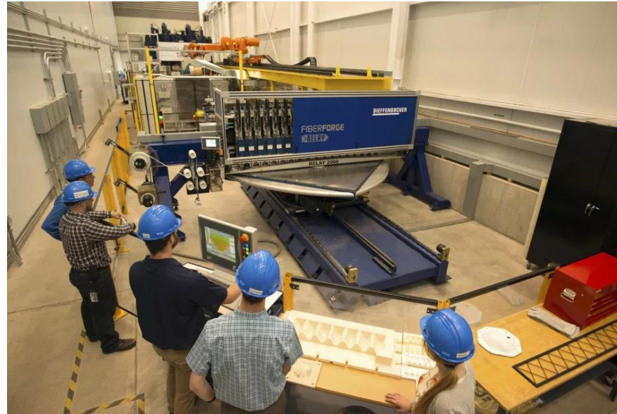
Automated Tape Layup Cell
