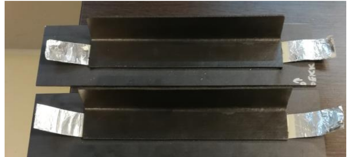
Pull-off Test Coupons
