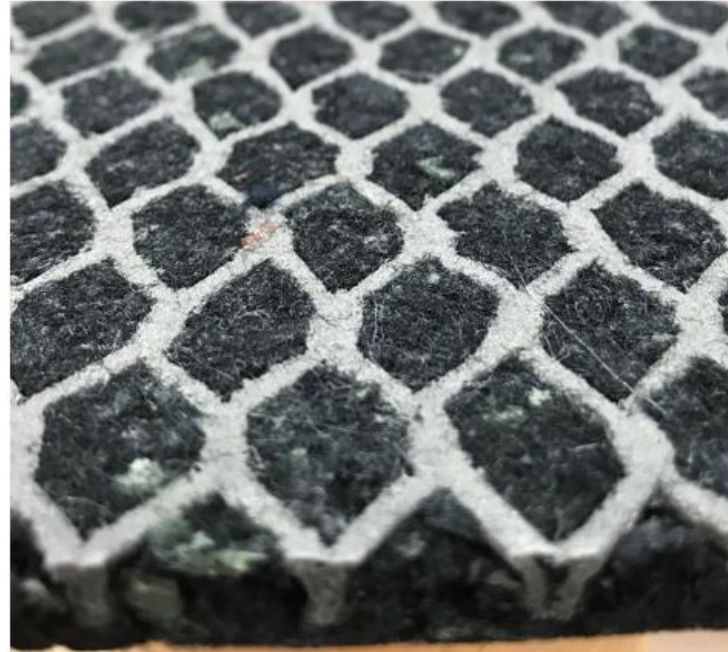
Hardfill waste fiber Honeycomb panel. Acoustic properties
