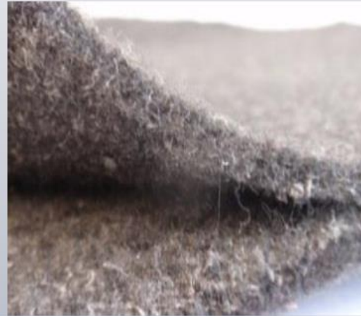
Recycled fiber layer between needle felts
