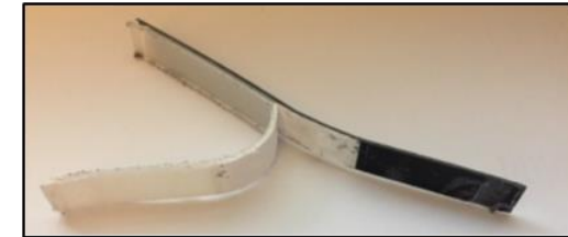
Adequate preheat Substrate Failure
