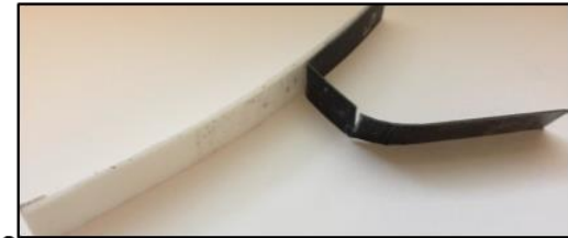
Low preheat Interface failure
