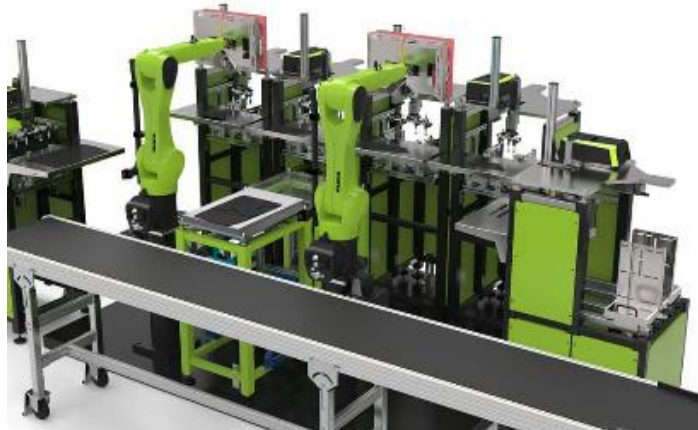
Organomelt – Tape Stacking Unit
