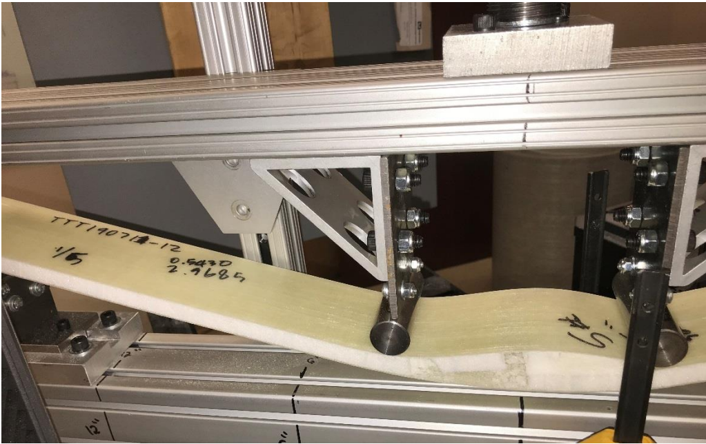
Compound failures due to extreme deflection
