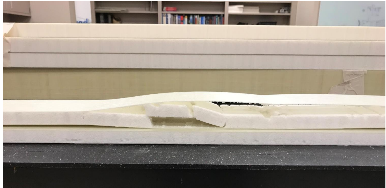
Compound failures due to extreme deflection
