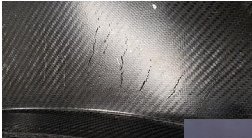
Fabric wrinkling due to inner flange compression - Credit - DARPA 2017
