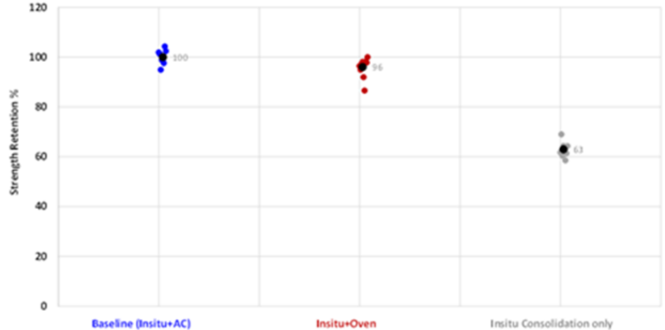
Percent Compression Strength Retention of PEEK LAFP Specimens manufactured using different processes (ISC+AC, ISC+OOA, ISC)
