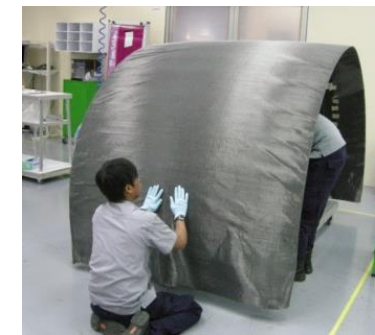
A320neo Fan Cowl Resin Film Infusion
