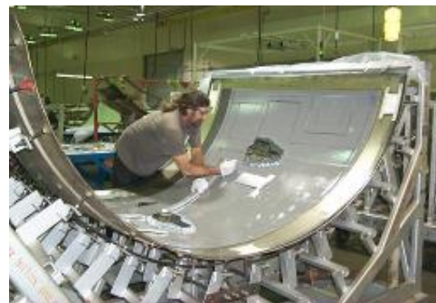
CF6-80C2 Fan Cowl Fully co-cured
