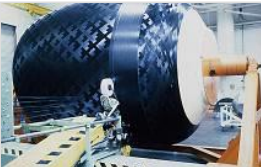
CF6-80C2 Fan Cowl Filament winding
