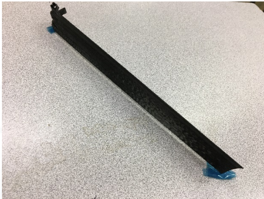
3D printed specimen Length: 250 mm (9.8")
