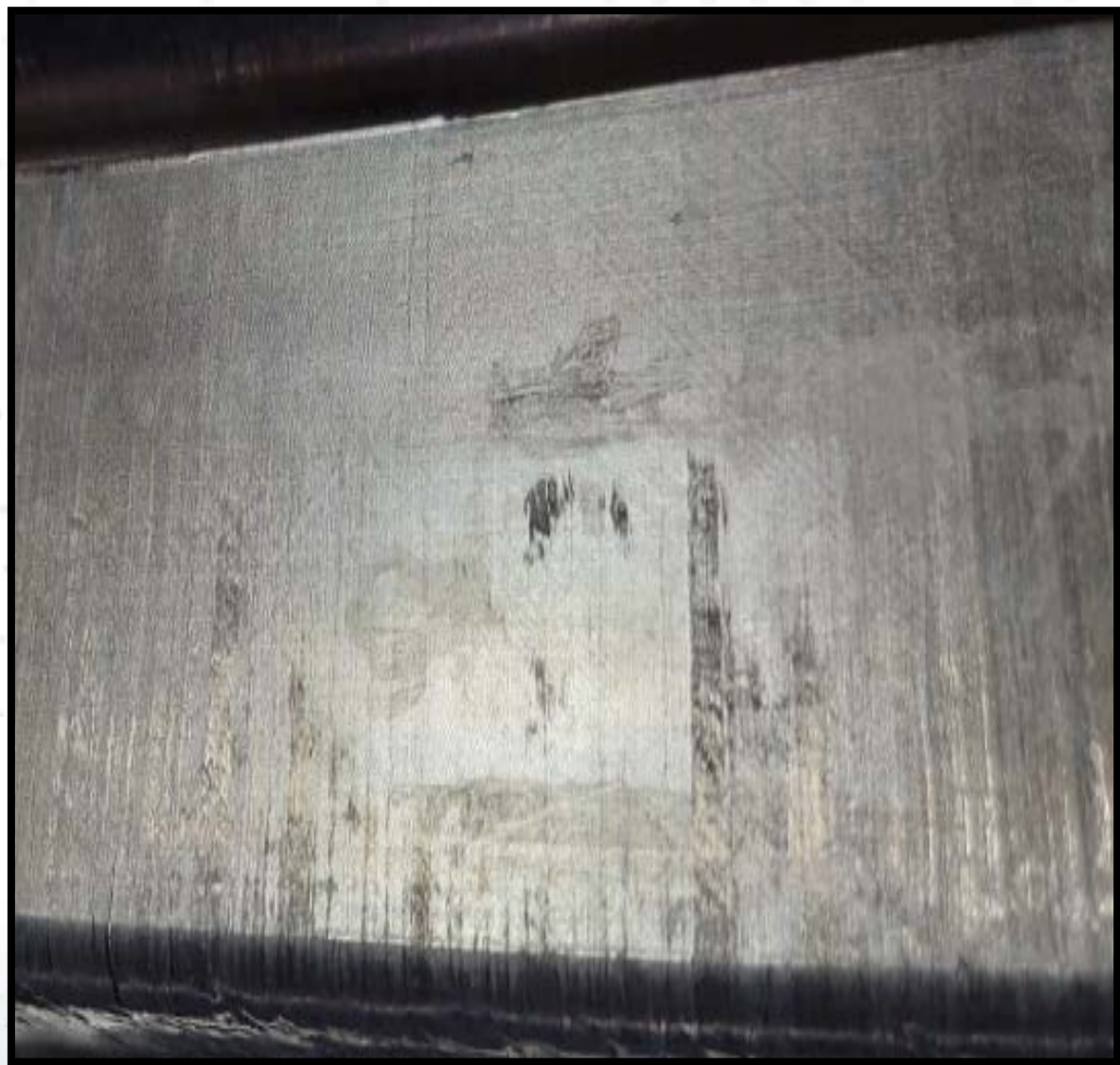
Frame after stamping. Good compaction on web after correcting blank alignment to dies
