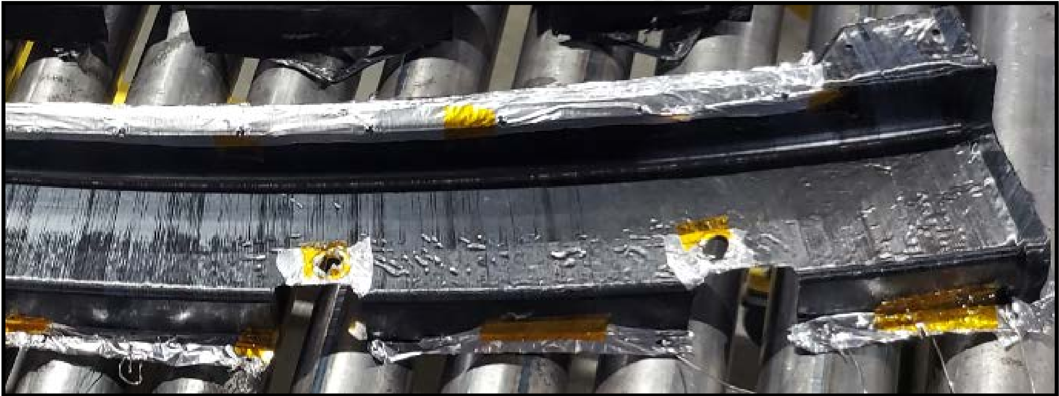
Day 1 frame after stamping. Significant wrinkling seen on web attributed to tool line up features preventing full tool closure
