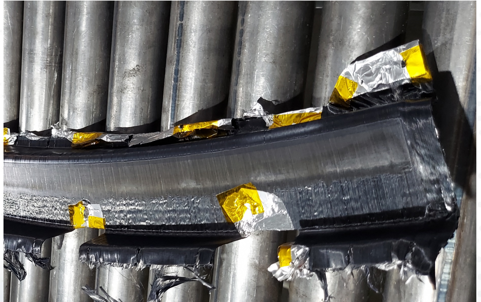
Frame after pressing – Full compaction in the thick part of the web
