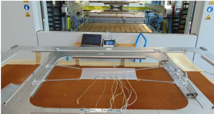
Fixation of skin in clamping frame
