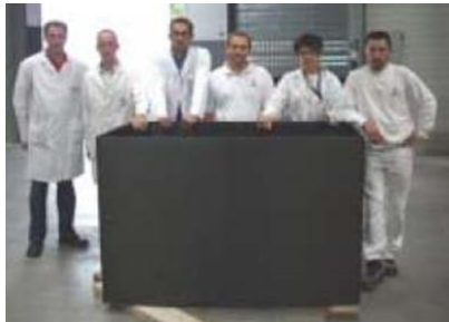
Maxi spring-back = 4 mm =>To be anticipated in future tool design
