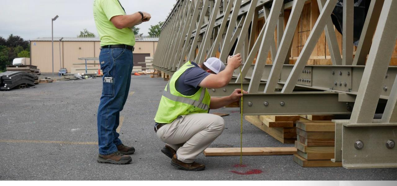
Deflection of 5 inches for test matched model of testing conditions/boundaries. Performed as intended and designed.
