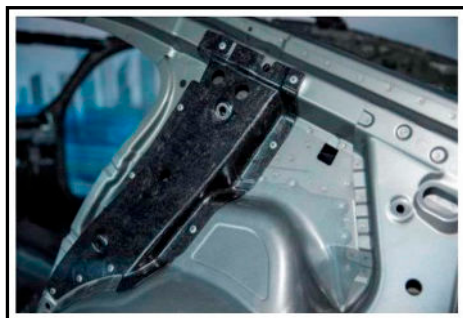
Figure 6. C-pillar from sheet molding compound (SMC, within BMW 7 series), reproduced from [157].
